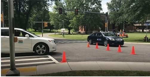
*Figure 3. A THEA vehicle (white car) waits as it receives an intersection movement assist warning being triggered by a New York City vehicle (black car) at the TFHRC test track. (Source: USDOT)*
